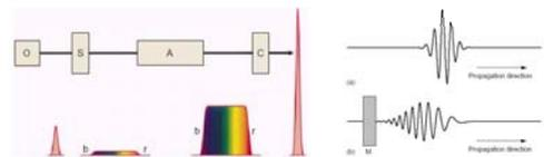
Figure 8 Diagram showing the principle of CPA. The oscillator output (O) is stretched in the grating stretcher (S) such that the red frequency components (r) travel ahead of the blue (b). The peak intensity is reduced in the process. The stretched pulse is then amplified in a regenerative or multipass amplifier (A) before recompression in a grating-pair compressor (C).
